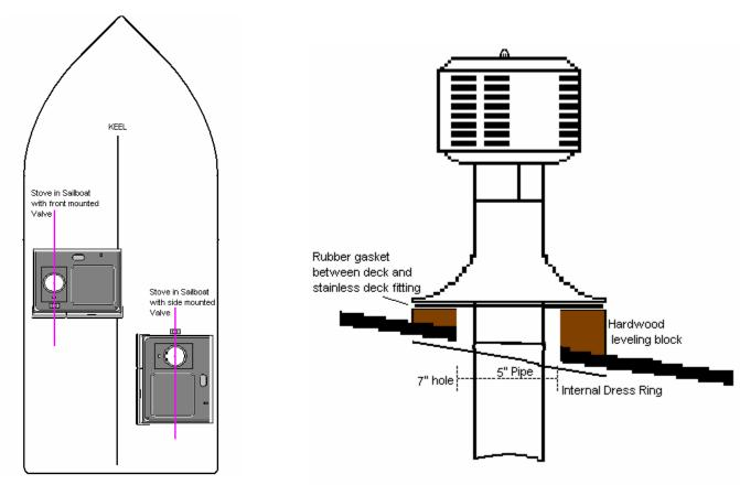
Note: Burner and valve are in line with the keel.
