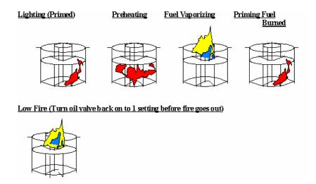
After start up and after a couple of minutes have passed, the flame should be lemon yellow, perhaps with some blue. Dirty orange colors or visible soot or smoke indicate an inefficient burn. The fan should be turned on or up to add more air in this situation or the valve turned down.
