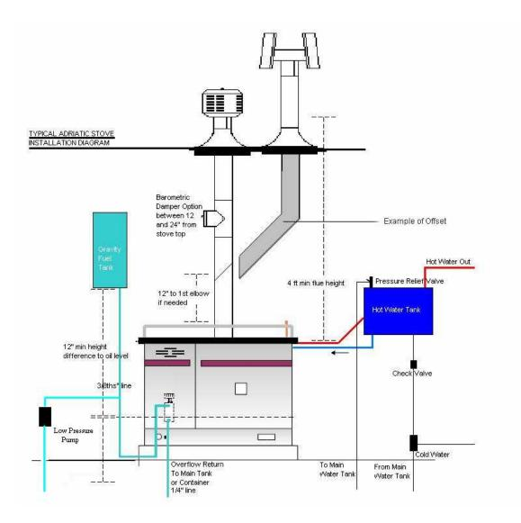
NOTE: Not all installations will require a pump, gravity tank, elbows, or coil options
