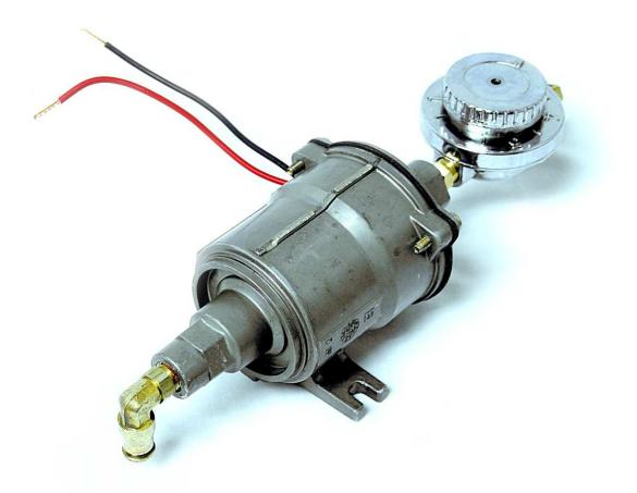
We recommend using an elbow fitting on the fuel inlet. When priming this pump hold down the knob of the pressure regulator to prime the fuel lines and take out the air then turn the dial to the lowest setting on the regulator and increase pressure 1 increment at a time until the pump is just delivering a small amount of fuel as the heater/stove only requires a very small amount .
