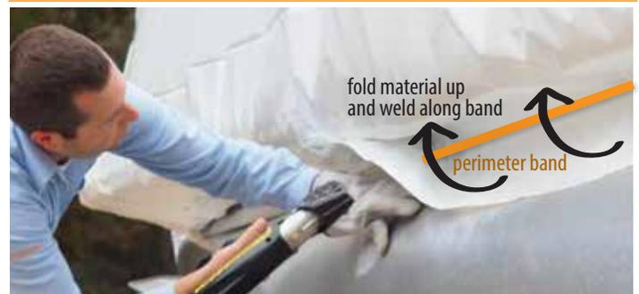
Instead of tucking the shrink wrap film under the perimeter band (like you would with a traditional recreational boat), **the shrink wrap should be put on the boat before the perimeter band strapping.** The perimeter band is then installed over the shrink wrap just below the decking. Once the perimeter band is tightened over the shrink wrap, fold the loose shrink wrap up and heat weld it over the exposed strapping.
