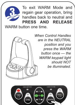
\* Normal system configuration will automatically activate WARM Mode every time the control system is started.
