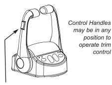
Toggle UP to trim engine drive unit in an upward position
