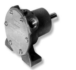
4. SELF-PRIMING – Primes at low or high speeds. For vertical lift of 10 feet (3.0mm), a minimum of 800 RPM is required. Pump will produce suction lift of up to 22 feet (6.7m) when wetted. BE SURE SUCTION LINES ARE AIRTIGHT OR PUMP WILL NOT SELF-PRIME.
