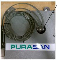
Install Dual Connector here, then plug Panel #1 and Panel #2 cables in as shown
