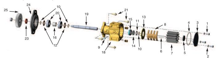
The following assembly/disassembly procedures apply to all 17000 Series pumps. Deviations from pump to pump are primarily a result of different methods of drive and mounting. Pump model numbers can be found stamped into the cover plate of the pump.
