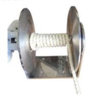
The chain / rope should be wound "thread lay", with close even winding throughout the length of the chain / rope. If wound unevenly, the turns of chain / rope bunch-up, cross wind and are liable to form doglegs, particularly on the more flexible chain / ropes.
