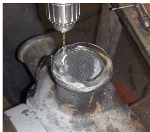
Figure 19-Remove Jig and continue Drilling  $\frac{3}{4}$ " Deep
