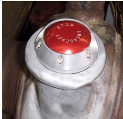
Figure 26-Finished E-Stop Switch Arrangement Installed into the Winch Horn.
