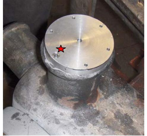
Figure 15-Horn Jig Inserted into horn center
