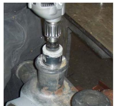
Figure 12-Drilling the horn center
