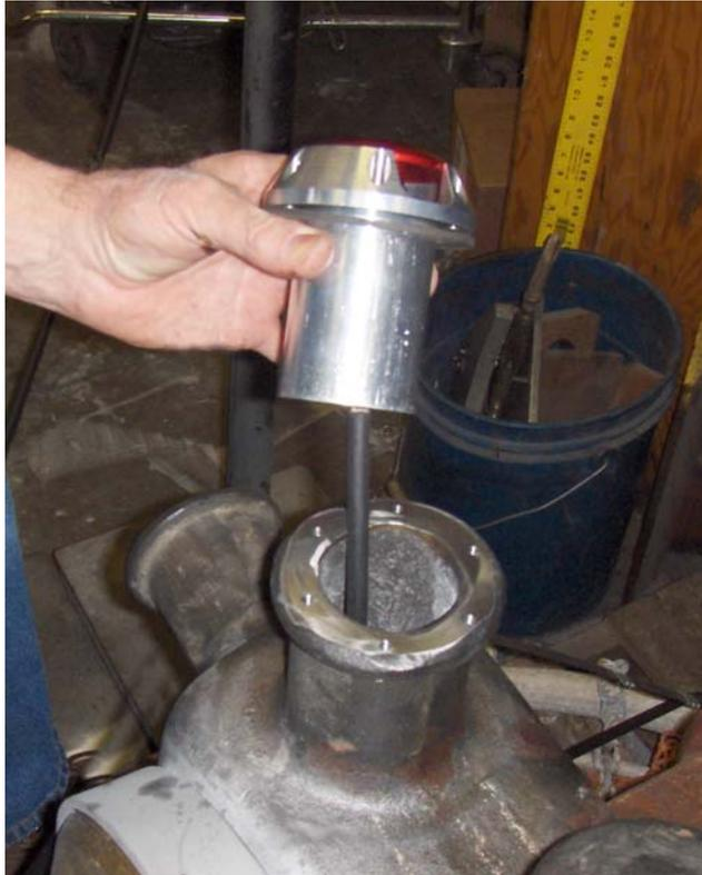
Figure 25-Inserting the E-Stop Arrangement into the Winch Horn.
