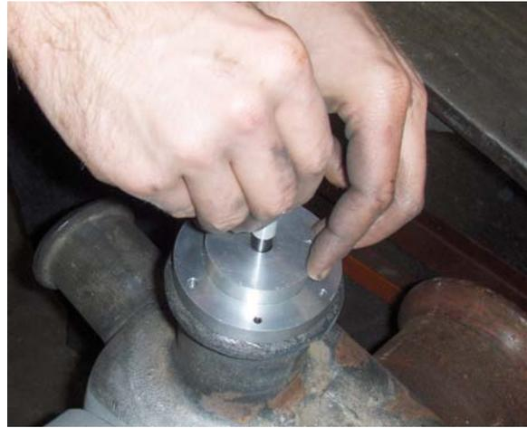
Figure 6-Marking the horn center
