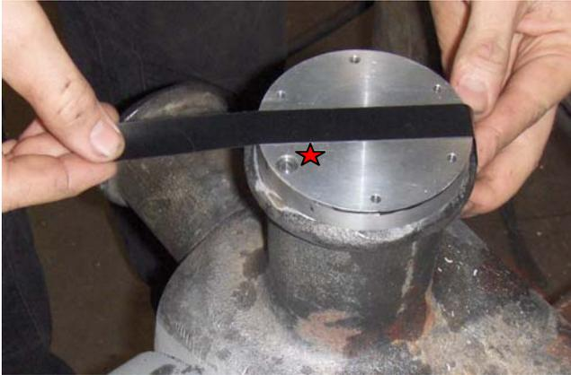
Figure 16-Secure Horn Jig to the horn
