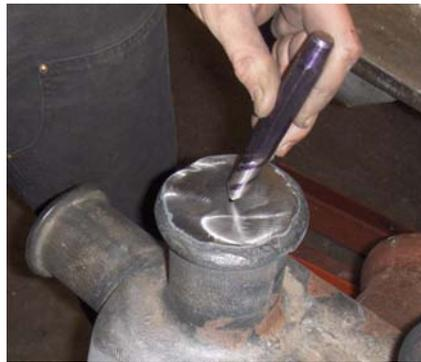
Figure 8-Preparing to Center Punch horn center
