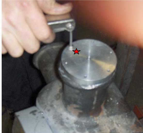
Figure 23-Secure Horn Jig to Winch Horn
