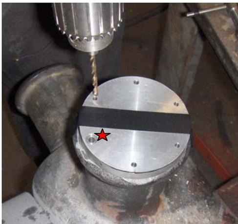
Figure 18-Drill 1st Mounting Hole into Jig to the horn
