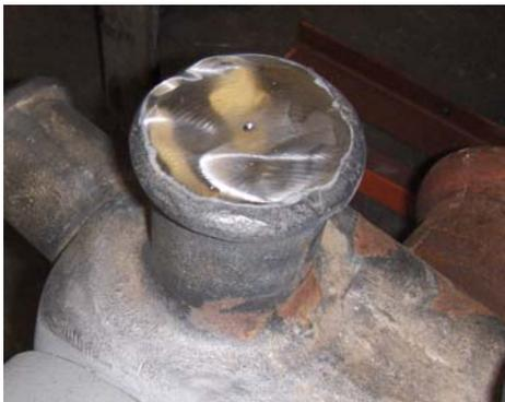
Figure 10-Horn center punched in center
