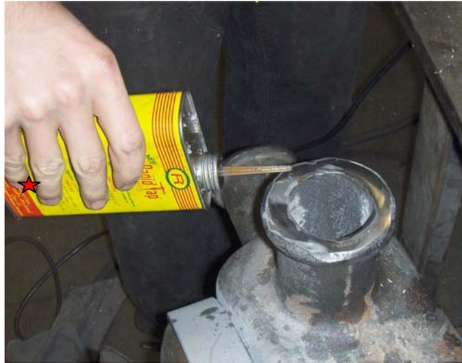
Figure 20-Apply Oil to assist in drilling 3/4" Deep
