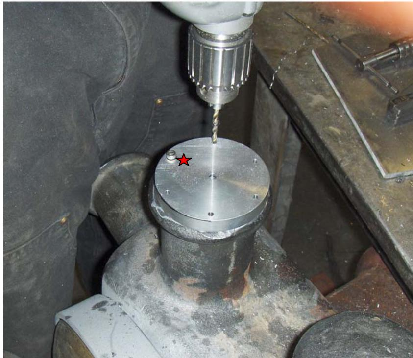
Figure 24-Drill remaining holes using secured Horn Jig
