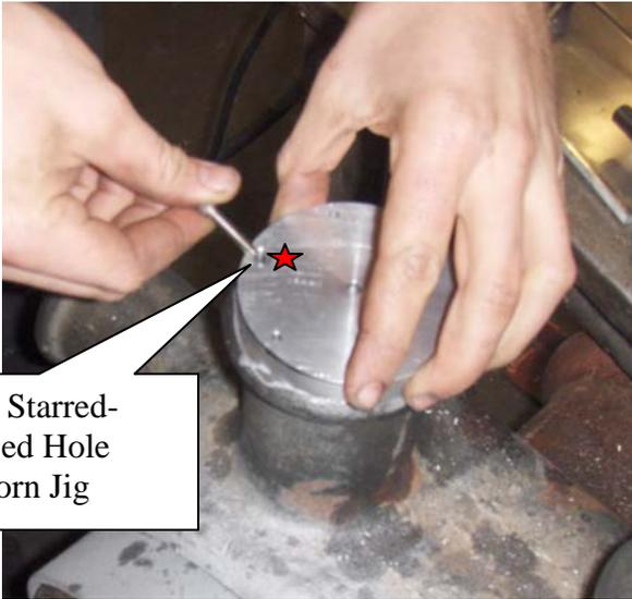
Figure 22-Special Recessed Hole over 1st Tapped Hole
