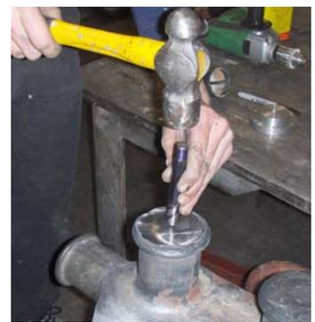
Figure 9-Center Punch the horn center
