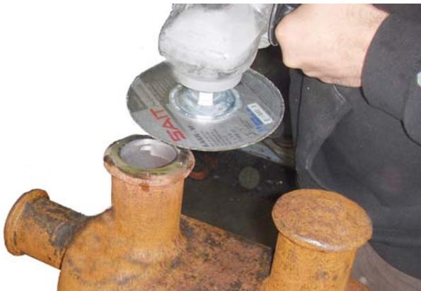
Figure 1-Grinding the Selected Horn
