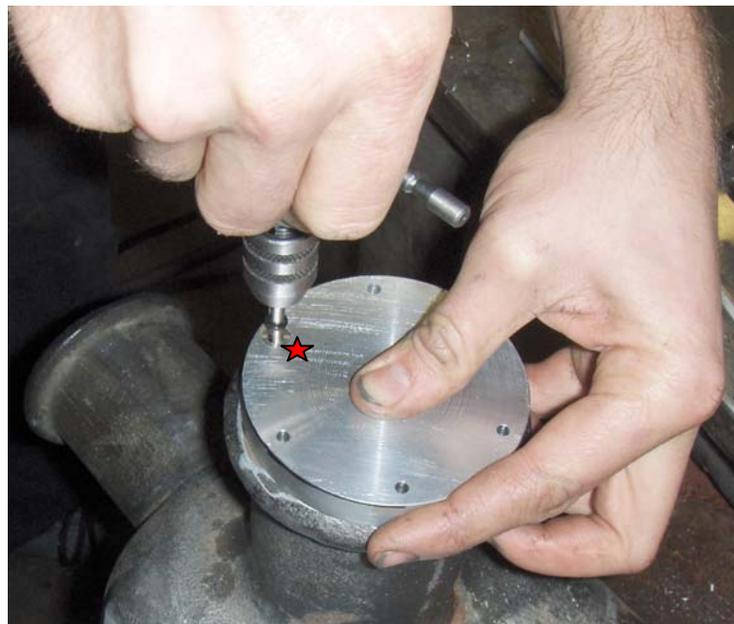
Figure 21-Tapping threads into Winch Horn using Horn Jig.
