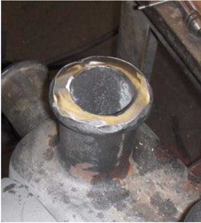
Figure 13-Horn center drilled out
