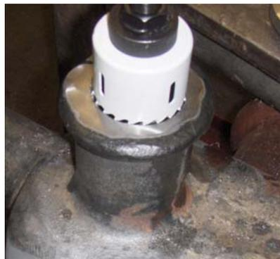
Figure 11-Preparing to Drill horn center
